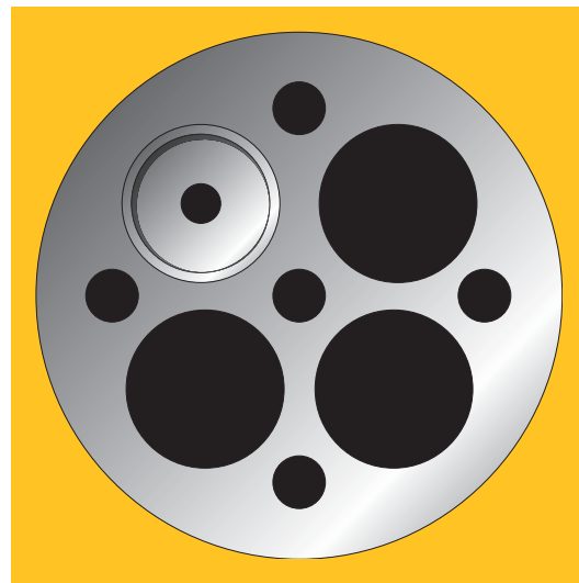
Multiple hole blocks can increase throughput by calibrating several probes simultaneously.
